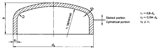
Designation of a cap in accordance with this standard, having an outside diameter,  $d_{a}$ , equal to 88,9 mm and a wall thickness,  $s_{1}$ , equal to 2,3 mm, made from material belonging to material group C as in DIN 2609 (C):
